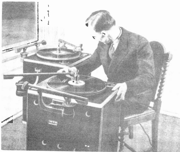
Fig. 2 Positions of transcription turntables and operator for running a transcribed program.
