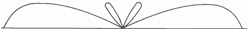
Fig. 38 The vertical radiation pattern of a five-eighths wave vertical antenna close to the ground.
