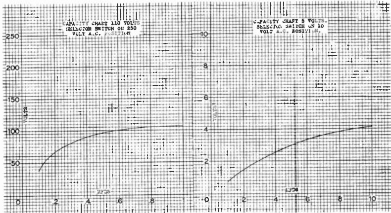
Fig. 20 Capacity-voltage calibration graph for Triplet Model 1200-A Universal Meter.
