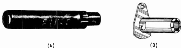
Fig. 21 (A) Picture of a modern fuse retainer. (B) Picture of an antenna receptacle.
