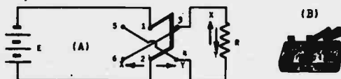
Fig. 4 (A) Double pole-double throw (abbreviated DPDT) switch circuit in which the direction of the current through resistor R may be changed by throwing the arm of the switch.
