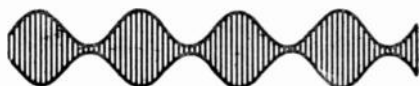
Fig. 17 Appearance of the oscillating current in a Hartley oscillator when being blocked with a high grid-leak resistance.
