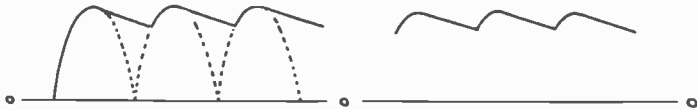
Fig. 42 The dotted line represents the output voltage of the rectifier, and the solid line the voltage across the first filter condenser C_1 . B shows the voltage across C_1 drawn separately.
