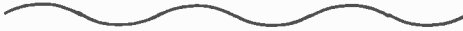
Fig. 43 Waveform of the current which flows through the first choke L_1 of Fig. 41.
