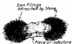
Fig. 1 Illustrating the attraction of Lodestone or Magnetite for Iron Filings.
