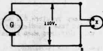
Fig. 35 If X is a voltmeter, it will measure the voltage output of the generator, but if it is an ammeter, it will quickly burn out, because AMMETERS MUST NOT BE CONNECTED IN PARALLEL.
