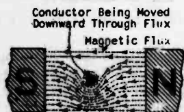
Fig. 7 illustrating Lenz's Law. Magnetic repulsion is encountered as the current-carrying conductor is moved through the flux.
