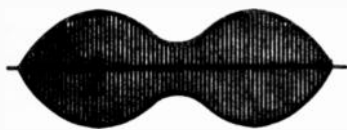
Fig. 18 Modulated R.F. voltage applied between grid and filament.
