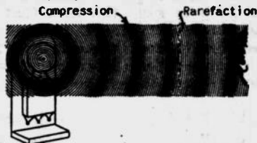
Fig. 12 Diagram illustrating the passage of sound waves through the air. The compression and rarefaction of the air molecules are indicated by the heavy and light lines respectively.
