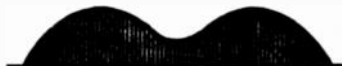
Fig. 19 Grid current pulses. Rectification occurs because grid current can flow in only one direction
