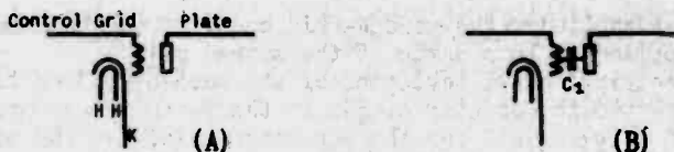
Fig. 3 (A) Elements in a triode tube. (B) C 1 indicates the capacity between plate and control grid.
