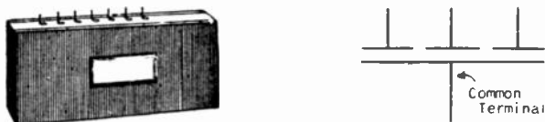
Fig. 23 (A) View of Condenser Bank. (B) Symbol for Condenser Bank.
