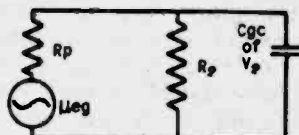
Fig. 12 Equivalent electrical circuit for the plate circuit of a direct-coupled amplifier.
