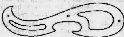
Fig. 7 Outline of a "French curve". This instrument is for the purpose of drawing a smooth curve through several points.
