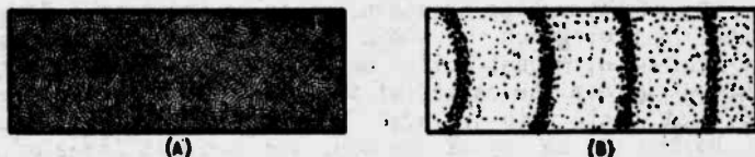
Fig. 3 (A) Normal air molecules. (B) Air molecules compressed and rarefied by sound waves.
