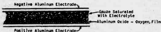
Fig. 14 Cross-Section of "Dry" Electrolytic Condenser.
