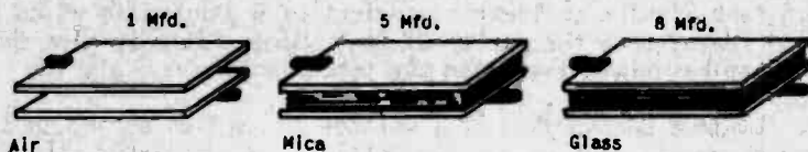
Fig. 7 Illustrating the Meaning of Dielectric Constant.
