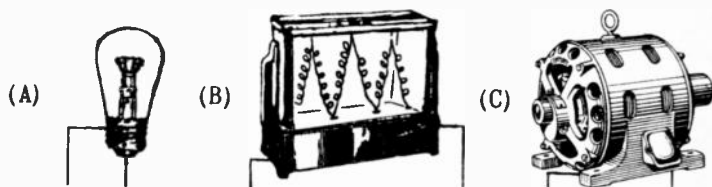
Fig. 9 Using the word "ampere". A current of .25 ampere passes through the incandescent lamp, 5 amperes pass through the element of the toaster, and 10 amperes run the electric motor.
