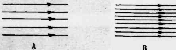
Fig. 10 (A) A Weak Magnetic Field. (B) A Strong Magnetic Field.
