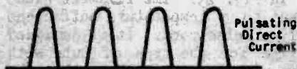
Fig. 24B Waveform of the current flowing through the load resistor of a half-wave rectifier.
