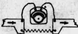
Fig. 8 A shunt connected across a meter. Only a part of the total current flows through the meter.
