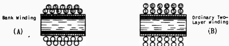
Fig. 13 (A) Bank winding used to minimize the effect of distributed capacity. (B) Ordinary layer winding in which the distributed capacity is large.
