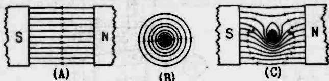
Fig. 8 Illustrating Lenz's Law. Flux between poles shown at A. Field around conductor shown at B. At C, both fields are combined.
