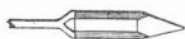
Fig. 10 An ordinary copper-tipped soldering iron. This type of iron must be heated over an open flame.
