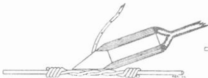
Fig. 15 (A) This illustrates the incorrect way of applying the iron and cored solder to the joint to be soldered.
