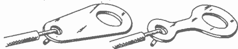
Fig. 25 This diagram shows how a wire should be connected to a solder lug before soldering.
