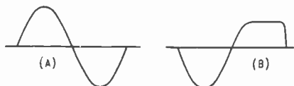
Fig. 9 (a) Wave produced when maximum undistorted power output of amplifier is exceeded.
