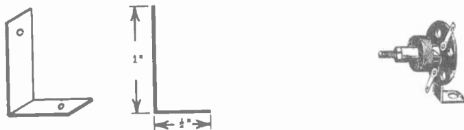
Fig. 9 Two views showing the construction and size of the special bracket needed to mount the R.F. choke. A view of the mounted choke is also shown.
