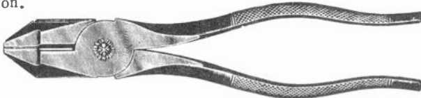
Fig.4 This type of plier is usually called lineman's side-cutting pliers. They are a heavy-duty tool used by electricians.
