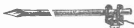
Fig. 27 A popular type radio ground rod. These ground rods may be purchased in lengths from three to six feet.
