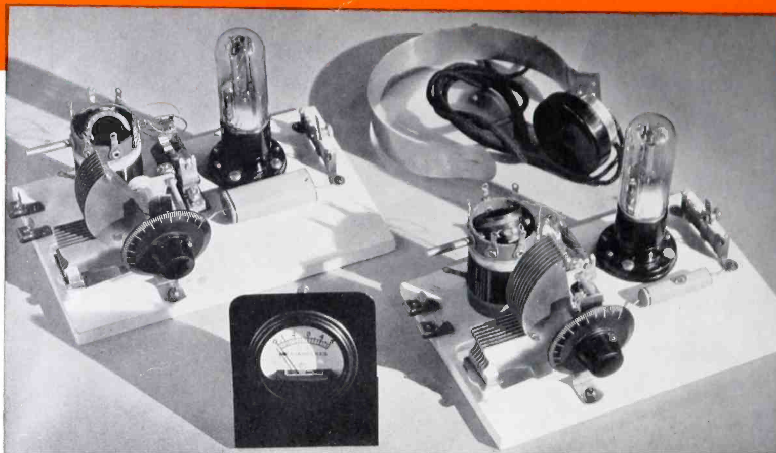
Above—Showing layout for test conducted with modulated oscillator and detector, Outfit No. 4
