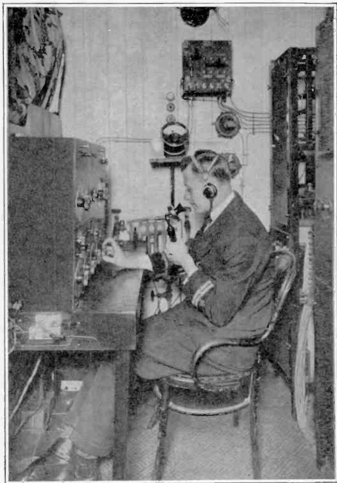
By means of this radiotelephone set, installed on the steamship "America," it is possible to talk and listen at the same time.
