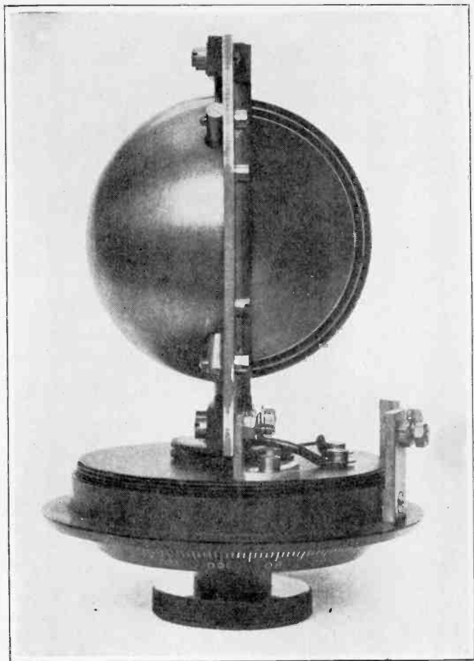
Another view of the British Government's ball condenser with one of its hemispheres partially turned.
