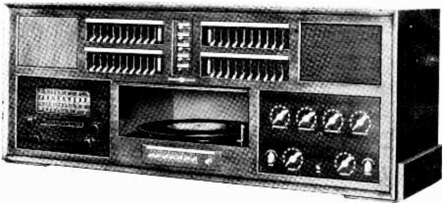
School sound system with radio, microphone, and phono input. By means of selector switches the sound can be distributed to the various rooms in a building.
