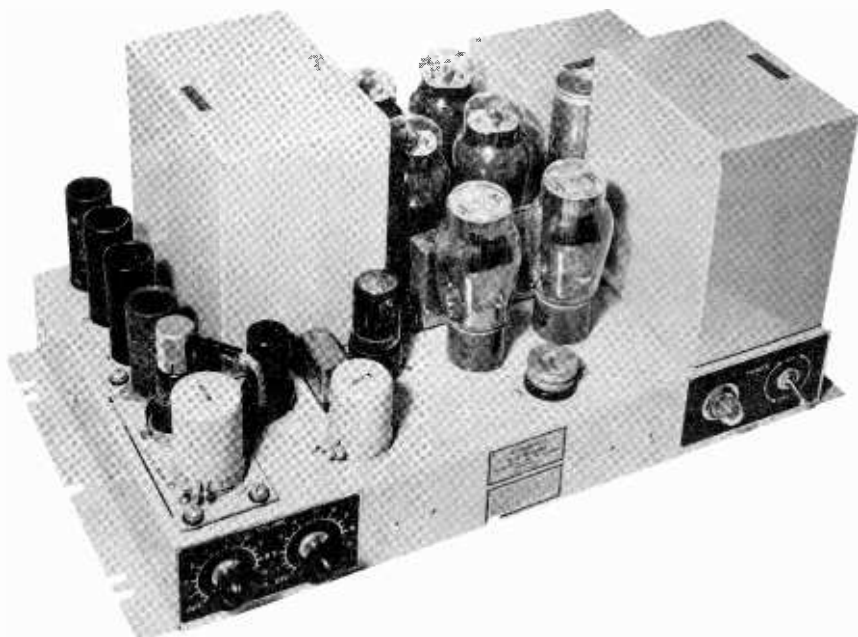
A 50-watt amplifier shown removed from cabinet.
