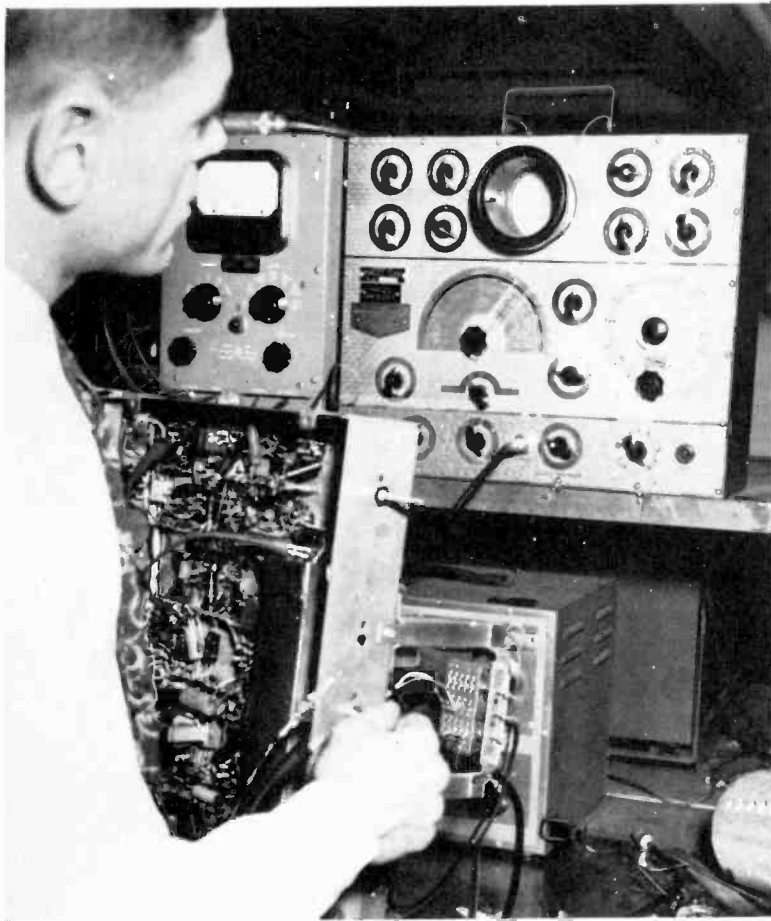
Philco precision visual alignment generator is shown here as it is used for adjusting the performance of an f-m receiver.
