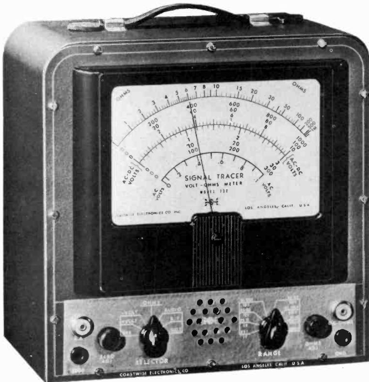
Modern signal tracer equipped with electronic volt-ohmmeter for visual observation, and permanent-magnet speaker for aural tests.
