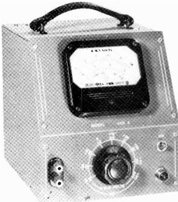
High grade vacuum-tube voltmeter designed and calibrated to read directly in rms values.
