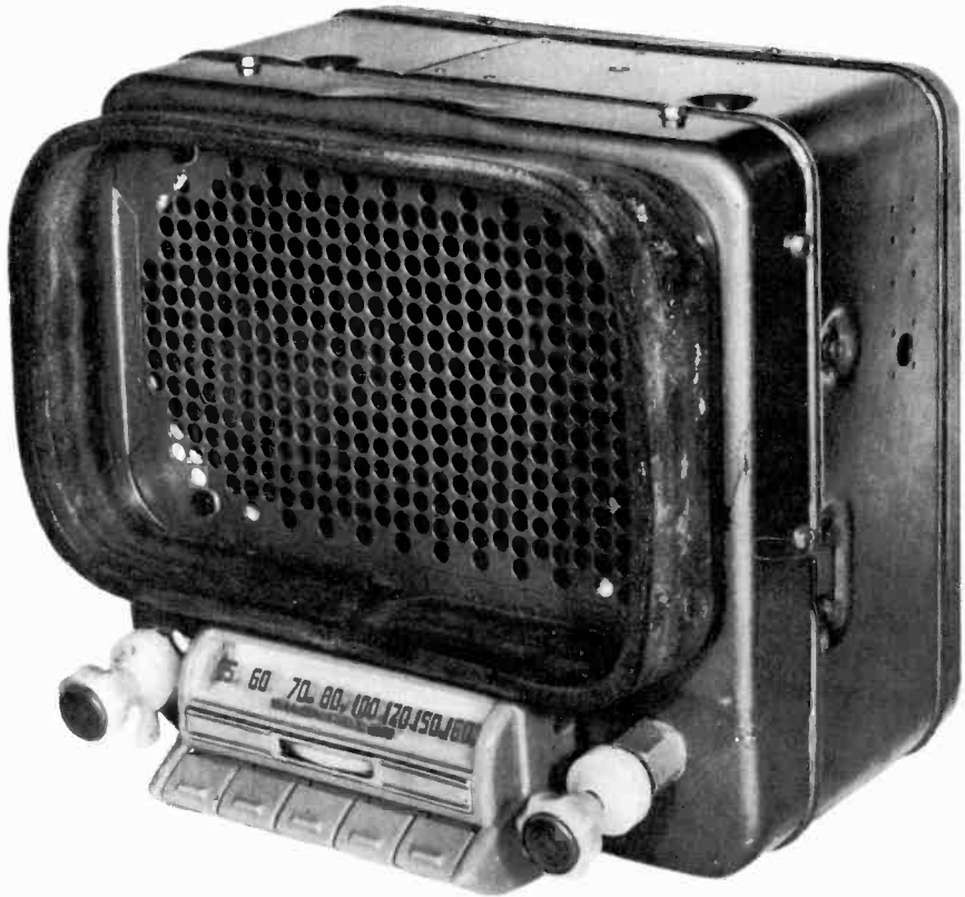
Auto radio receiver equipped with 5-button automatic station selector.
