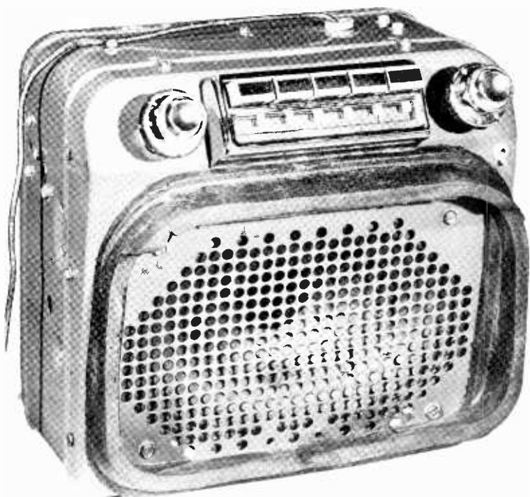
Complete auto radio receiver as used in Oldsmobile cars.
