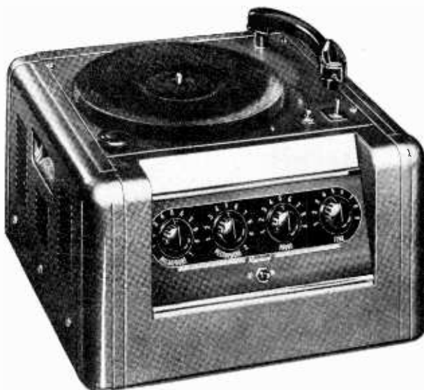
P-A unit equipped with phonograph turntable. The panel contains two microphone input controls, a phonograph input control, and a tone control.
