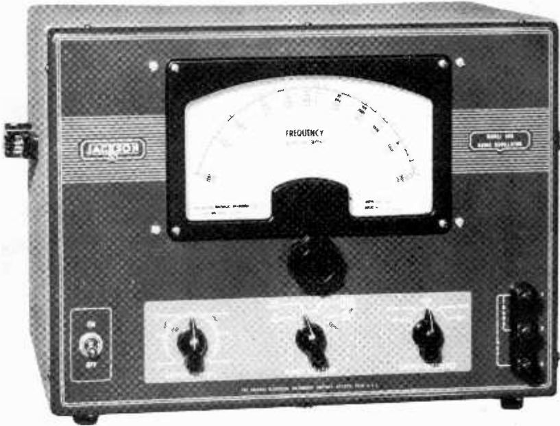
Audio oscillator such as can be used for checking the frequency response of an audio amplifier.
