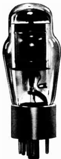
Fig. 1. A glow tube used for automatic voltage regulation.
