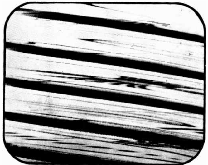
Fig. 2. This indicates horizontal sync trouble.
