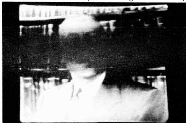
Fig. 3. A 60-cycle hum voltage causes one horizontal dark bar with brighter areas above and below, or might cause one complete bright bar between dark areas.
