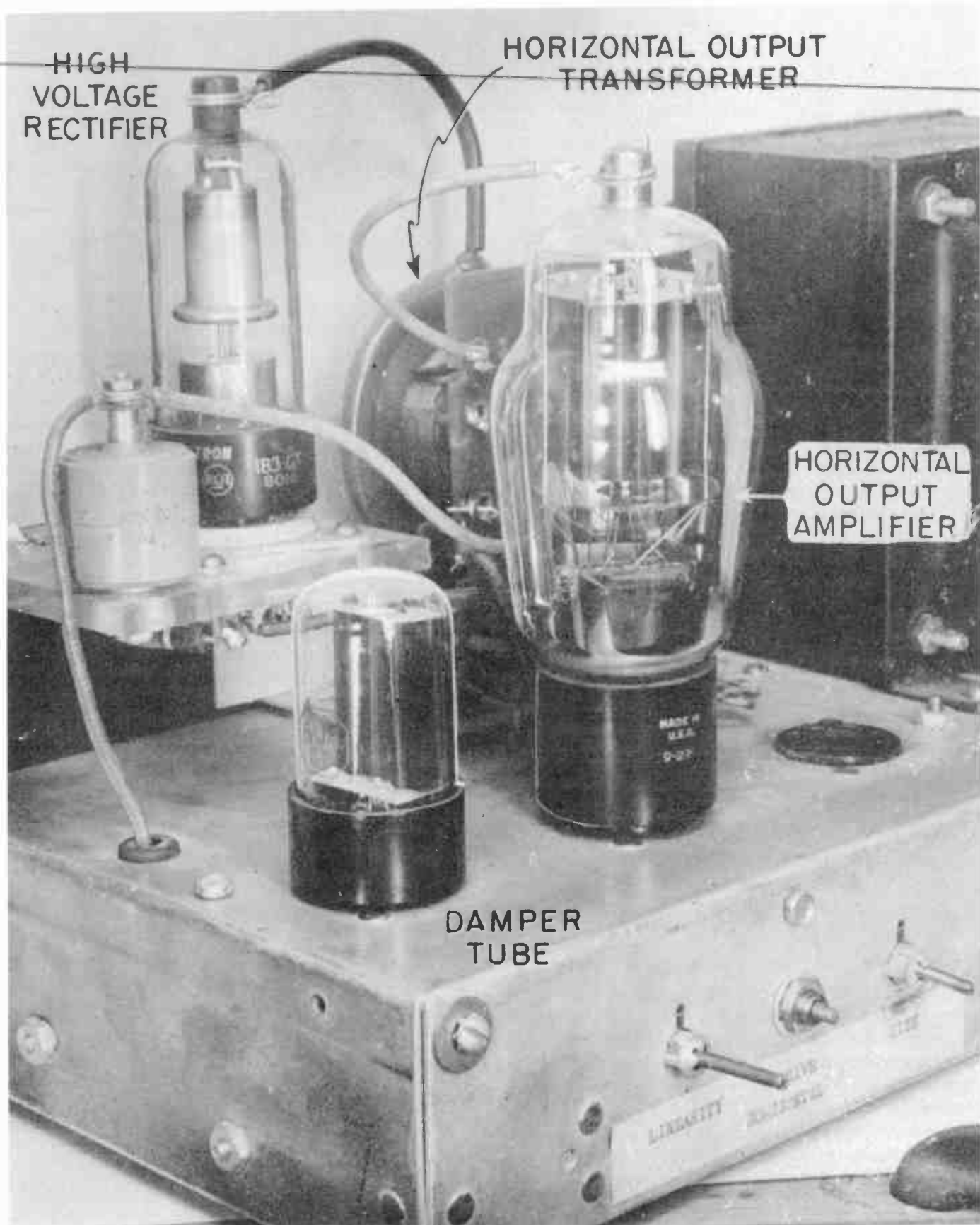
Fig. 1. The tubes and transformer of a horizontal deflection system and high-voltage power supply.
