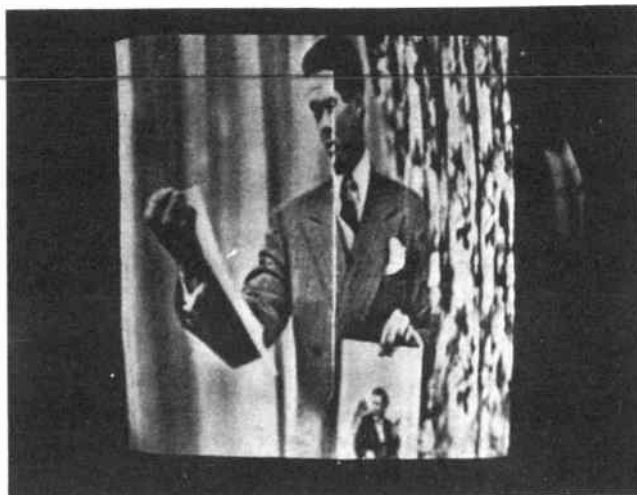
Fig. 11. Open or disconnected damper capacitors may cause this kind of foldover.
