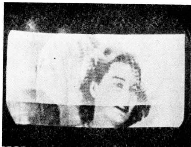
Fig. 10. This is a vertical fold.
