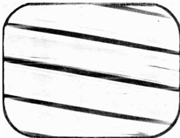
Fig. 15. These are not sound bars, they are due to lack of horizontal sync.
