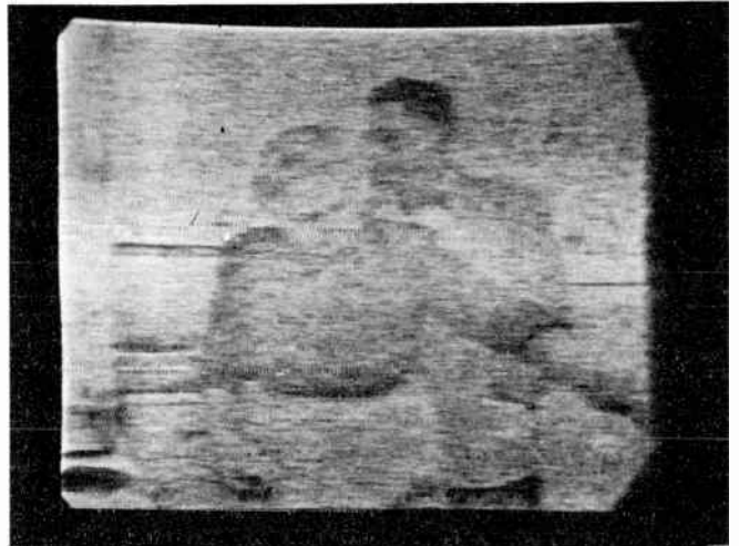
Fig. 7. The effect called snow results chiefly from thermal and tube noises, which become more apparent when received signals are weak.
