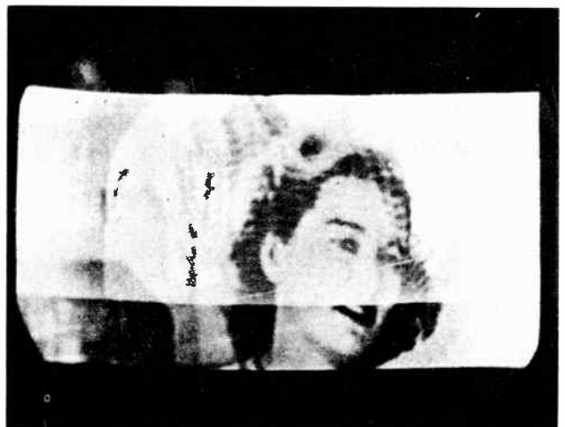
Fig. 20. Excessively high vertical sweep frequency may cause this effect.
