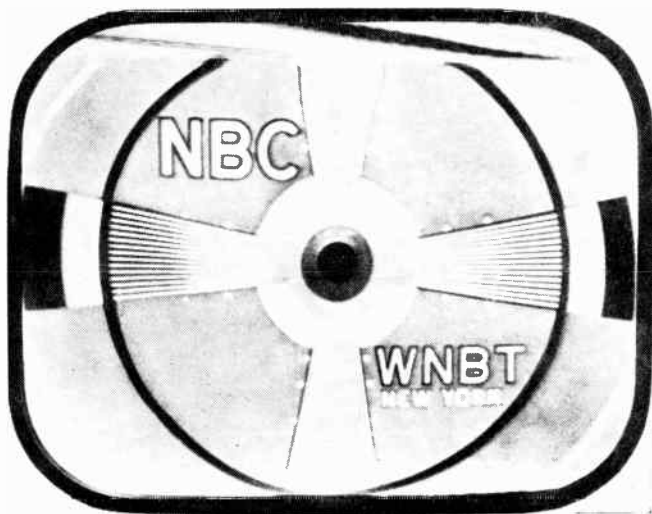
Fig. 11. Tear out occurs during momentarily failure of horizontal sync.
