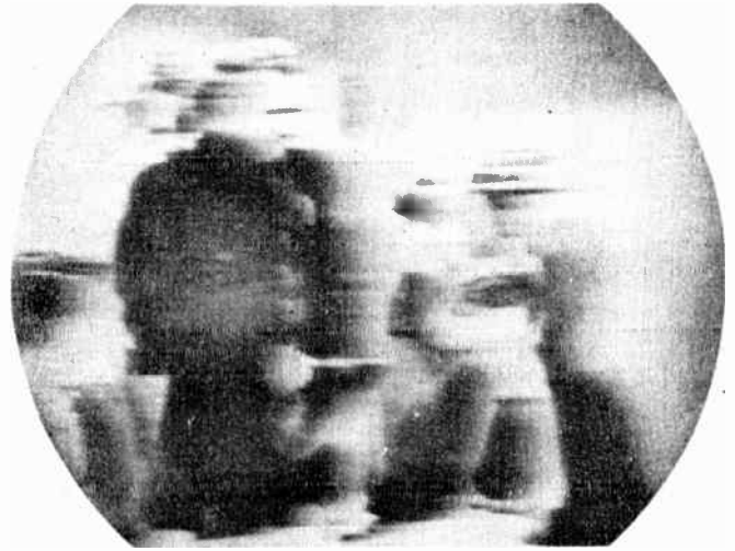
Fig. 11. Bad smearing, with long trailers.
