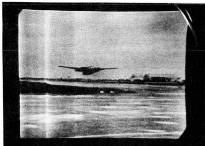
Fig. 20. Alternate light and dark vertical bands denote poor damping.
