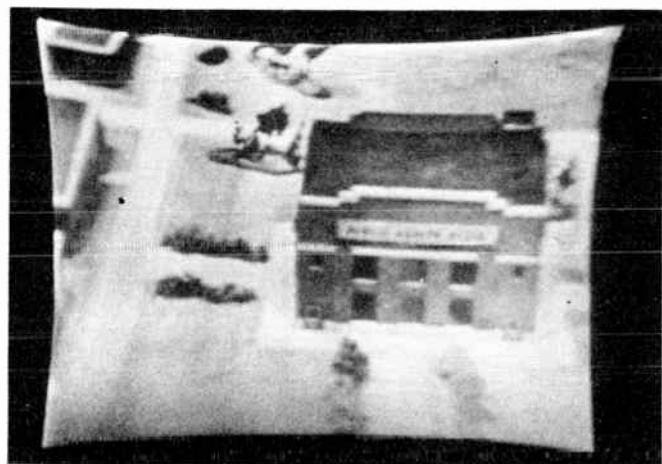
Fig. 26. This is called the pincushion effect.
