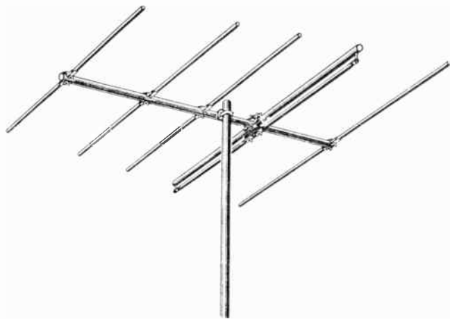
Fig. 13. A five-element Yagi antenna.
