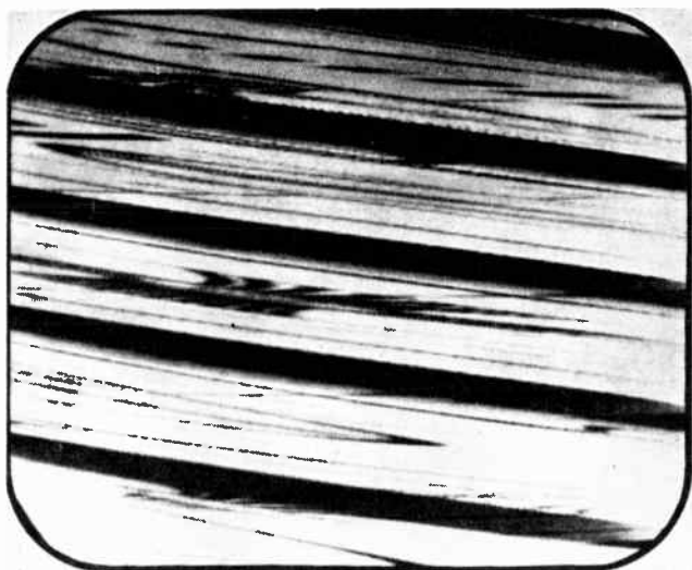
Fig. 21. The picture tube screen appears this way just before there is horizontal synchronization or lockin.
