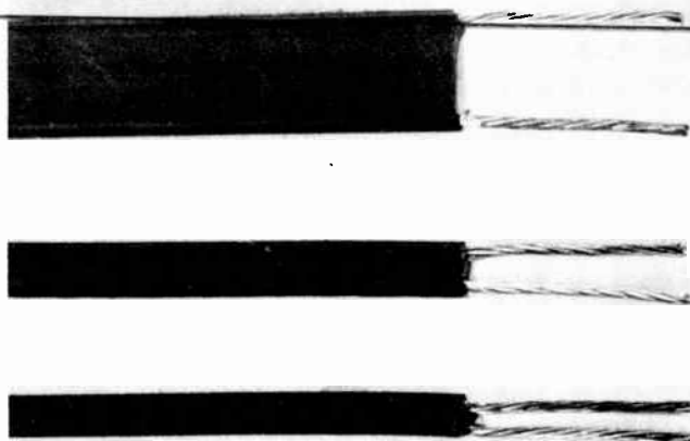
Fig. 3. Flat or ribbon types of transmission line with conductors molded in flexible insulations.
