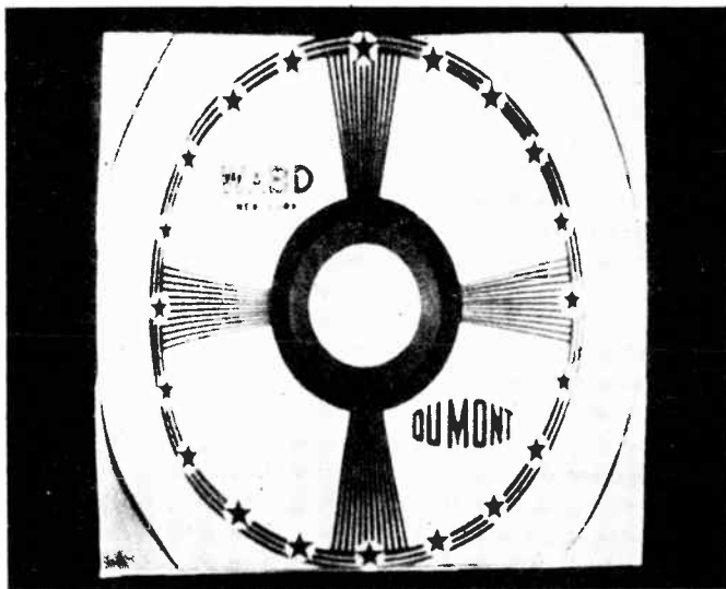
Fig. 16. Pictures are too narrow when the electron beam has insufficient sweep.
