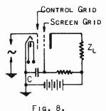
ODE. ELECTRIC LINES OF FORCE EXTENDING FROM THE CON-TROL GRID TOWARD THE PLATE TERMINATE ON THE SCREEN GRID WHICH, SO FAR AS THE R.F. VOLTAGE IS CONCERNED, IS AT CATHODE OR GROUND POTENTIAL. ELECTRIC LINES OF FORCE EXTENDING FROM THE PLATE TOWARD THE CONTROL GRID ALSO TERMINATE AT THE GROUNDED SCREEN GRID; THUS THERE
