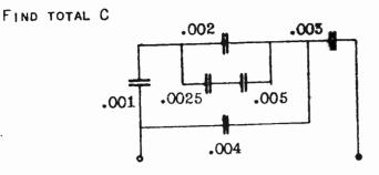
The equivalent capacity of the .0025 and .005  $\mu F$  condensers in series is:
