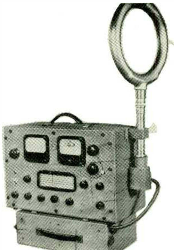
Fig. 24. —RCA Type 308-A Field Intensity Meter. Available with either a storage battery and vibrator type regulated power supply or dry battery box. The latter type is shown with the battery box below the meter.
