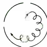
Fig. 38.—If magnetic field is increased above the critical value, electrons gyrate very rapidly.
