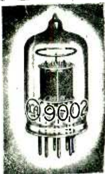
Fig. 10.—U.H.F. midget tube and socket arrangement.
