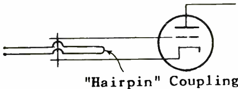
Fig. 33.—Method of coupling to a two-wire transmission line by means of a loop.
