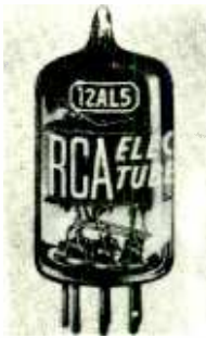
Fig. 20.—Photograph and base diagram of a 12AL5 miniature twin diode.
