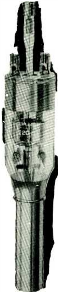
Fig. 8.—Type 220B—Filamentary water-cooled triode.
