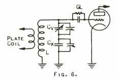
A preliminary calculation for  $C_X$  can be made on the assumption that  $C_X$  is large compared with the minimum value of  $C_V$  so that at a minimum setting of  $C_V$  the total circuit capacity C is not greatly decreased by the addition of  $C_X$  in series. Assume that with
