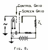
SCREEN GRID CONNECTS DIRECTLY, THROUGH A LARGE BYPASS CONDENSER, TO THE CATH-
