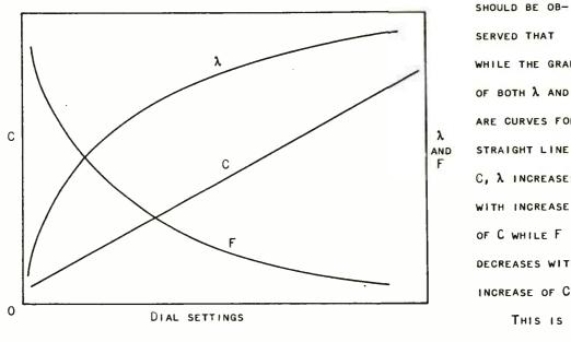
SERVED THAT WHILE THE GRAPHS OF BOTH  $\lambda$  AND F ARE CURVES FOR STRAIGHT LINE C, & INCREASES WITH INCREASE OF C WHILE F DECREASES WITH INCREASE OF C. THIS IS IN ACCORDANCE WITH
