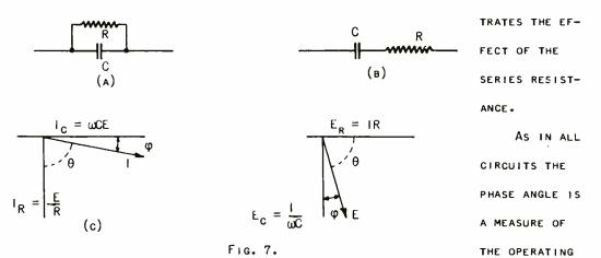
EFFICIENCY OF A CONDENSER AS IT EXPRESSES THE POWER-FACTOR OF THE CONDENSER. However, in well designed condensers operated under normal conditions the phase angle is so near  $90^{\circ}$  that it is difficult to express and handle in terms of Tan  $\theta$  as in other electric circuits. Thus the term "Phase Difference" is normally
