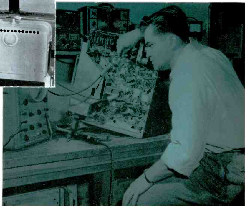
(Right) Serviceman is shown checking vertical sweep voltage generator in Television receiver. The waveform is checked step by step until the defect is located. Large numbers of different wave forms are encountered in television and the technician must be thoroughly familiar with each.
