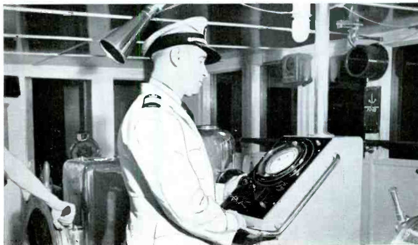
"Electronic Navigator" that sends out radar impulses to detect obstacles in path of a ship as far as thirty miles away. Instrument indicates land masses, other ships, lighthouses, buoys, even though natural vision is severely limited. (G-E Photo)
