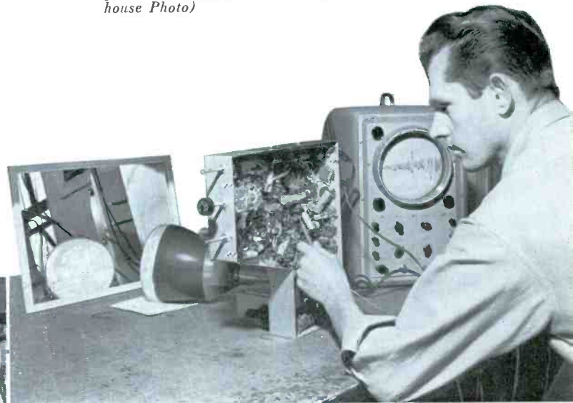
Trouble shooting on Television receiver. Circuits are complex and many misadjustments that would be relatively unimportant in standard broadcast receivers can completely spoil the operation at Television and FM frequencies.
