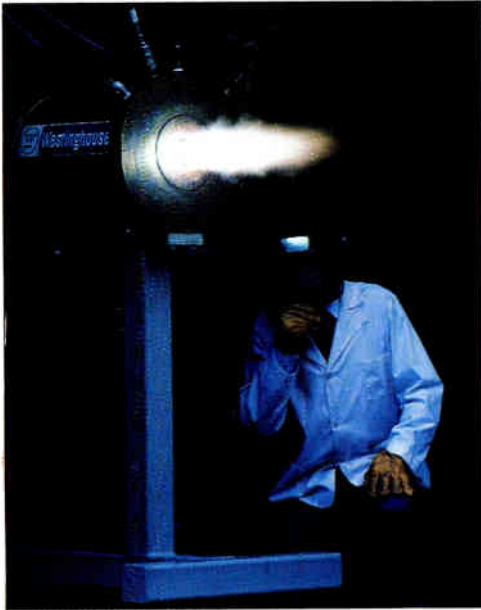
Plasma technology is being used in many industrial processes as well as in a new method for destroying hazardous liquid wastes. The Westinghouse Plasma System achieves destruction efficiencies in excess of 99.9999 percent on concentrated hazardous wastes.
