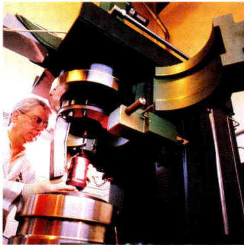
2—Finished GaAs boule ready for slicing and polishing into 3-inch wafers.
