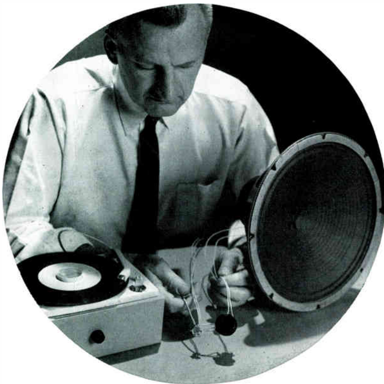
A molecular electronic function block as audio amplifier in a conventional phono system. Frequency range is 0 to 20 000 cycles, output is 5 watts when heat sink is used. Amplifier is at right in black mounting. At left is a molecular electronic preamplifier.
