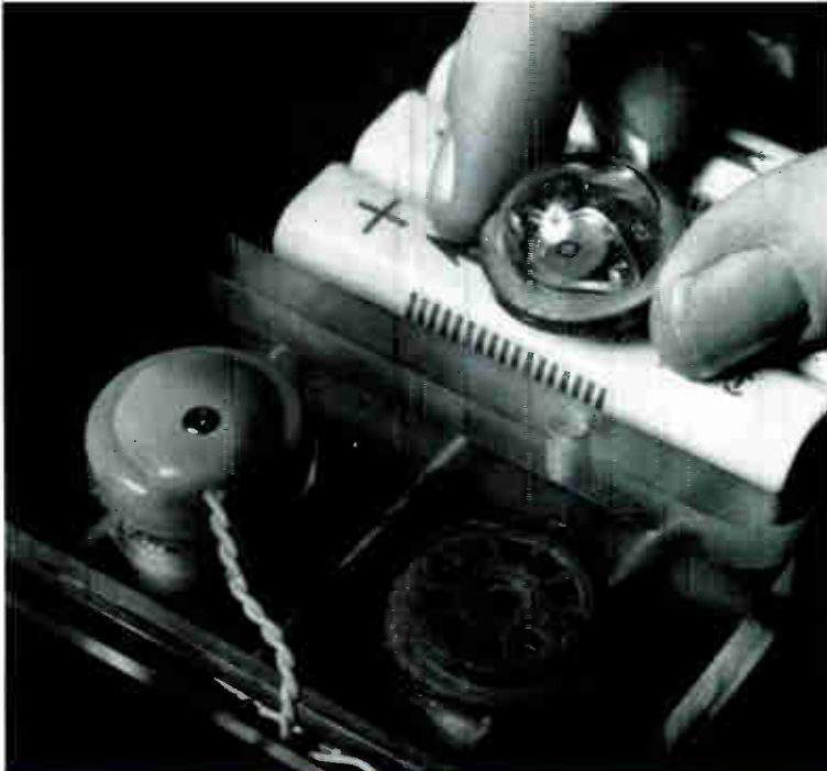
Fig. 2a—Light telemetry subsystem in which a single light-responsive monolithic element delivers an output whose frequency is measure of light intensity.
