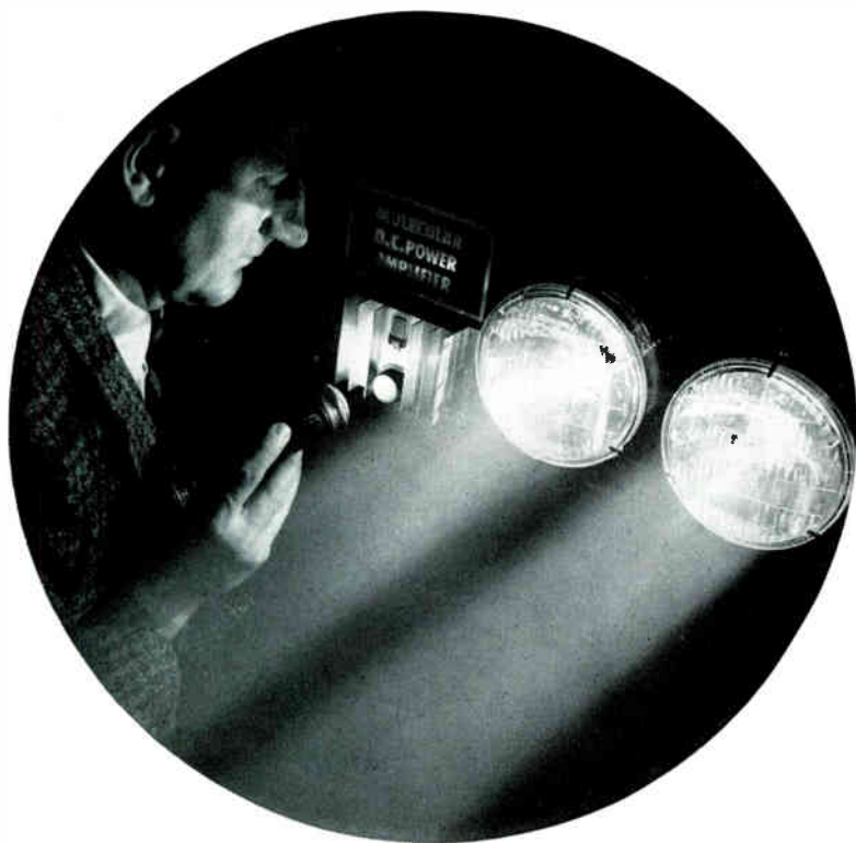
Demonstration of high-level amplifier as a dc amplifier. Intensity of light impinging on solar cell is fed to function block as dc signal voltage. Supplied from battery, function block amplifies signal and delivers matching dc output to head lamps.
