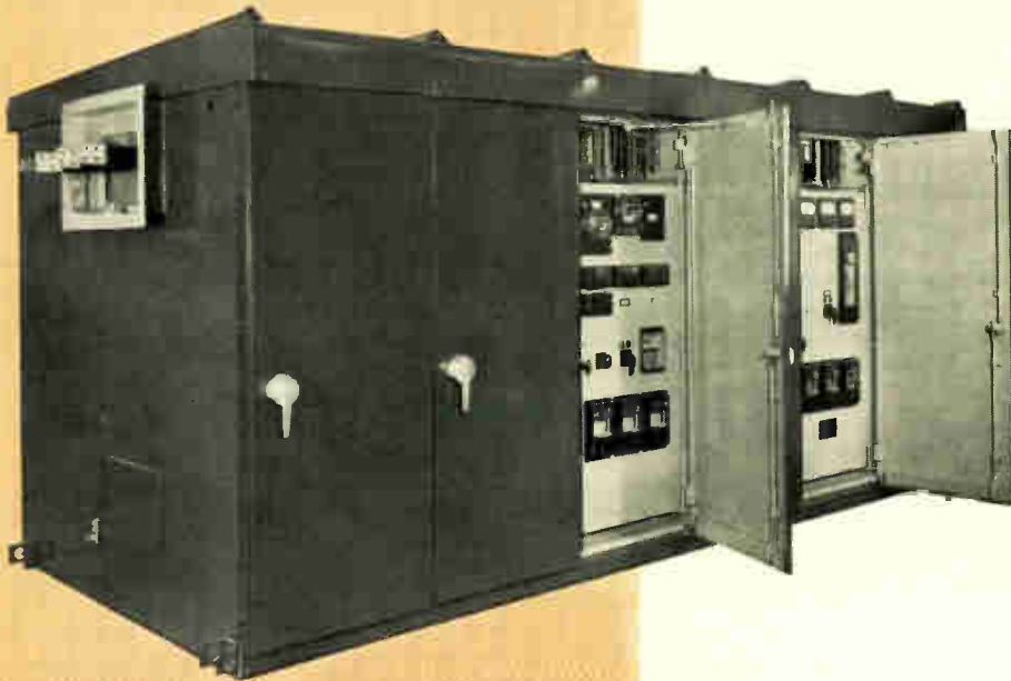
← A completely factory-assembled switchgear installation ready for packing and shipment. At the left is the throat for connection to the transformer. The exposed panel at left is a standard network control panel for the transformer breaker. The exposed panel at right is equipped with standard feeder-reclosing equipment. The two sections at the right house the auxiliaries.
