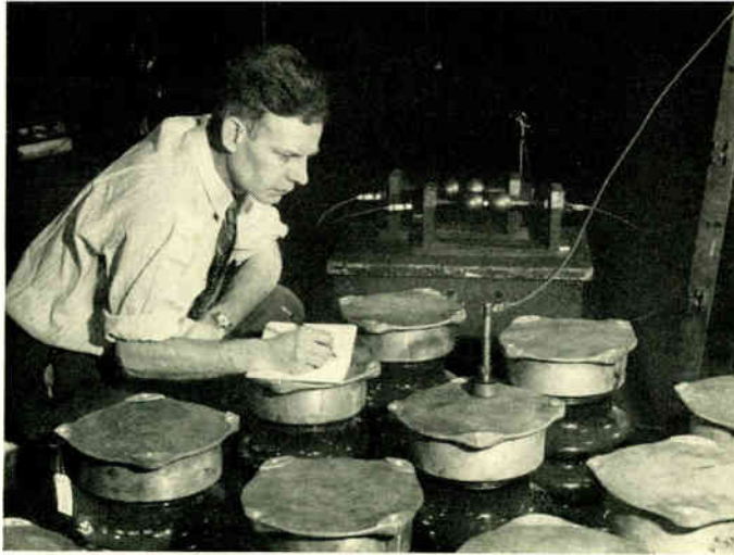
Testing SV lightning arresters for rotating machines.
