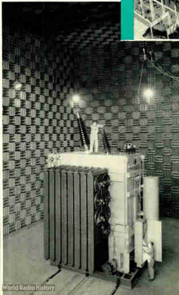
Two components, shown in the model above, are the surge voltage generator (left) and the anechoic vault.
