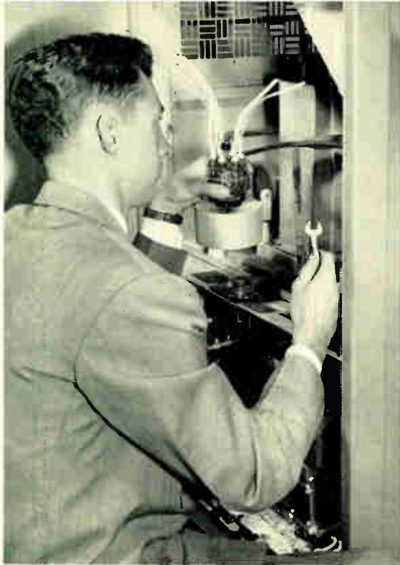
This industrial r-f generator tube has been redesigned for more convenient installation (see story below).
