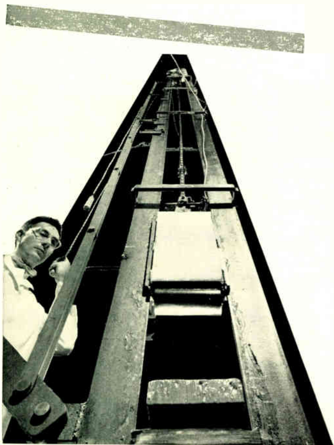
This guillotine tests shock resistance of metals.
