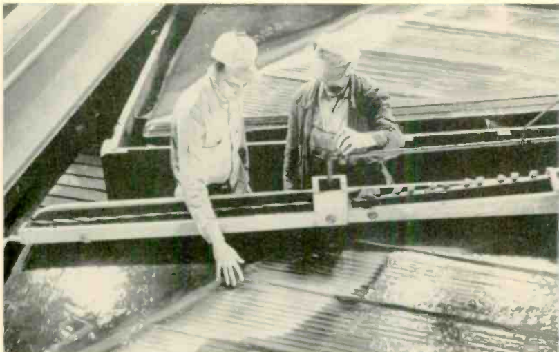
BY-PRODUCT. Iron pyrite is separated by flotation from the mineral mixture taken from a spiral classifier. The remaining material is treated on these vibrating tables for separation of tungsten and tin.
