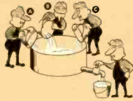
Fig. 5—The AND function is here represented schematically (left) and by an artist's sketch (above). An output occurs only when all the inputs are received.
