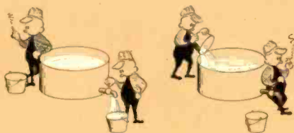
Fig. 7—The NOT element, unlike the AND and OR functions, delivers an output only when it does not receive an input, as depicted in the sketches above.
