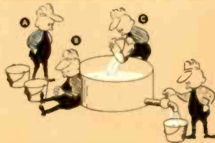
Fig. 6—The OR element delivers an output when any one of inputs A, B, or C is received. In the example, the output is caused by the existence of input C.
