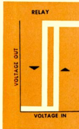
Fig. 1—An analog system gives a continuous signal, whereas the digital system provides a discontinuous, discrete signal. Simple examples are illustrated here.
