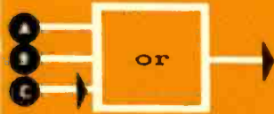
Fig. 6—The OR element delivers an output when any one of inputs A, B, or C is received. In the example, the output is caused by the existence of input C.
