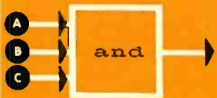
Fig. 5—The AND function is here represented schematically (left) and by an artist's sketch (above). An output occurs only when all the inputs are received.
