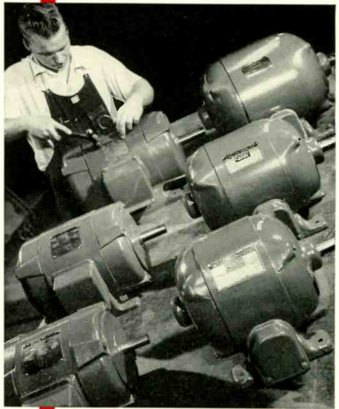
Comparison of the new Life-Line A motors (left) with type CSP. Top to bottom: 10 hp, 5 hp, 2 hp.
