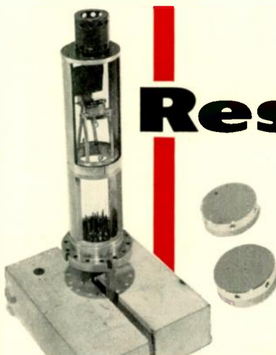
Left, low-temperature stage, showing single crystal copper target and ultra-black absorber mounted in place. Discs at right are enlarged view of copper target. Below, a view of the upper end of the test apparatus.
