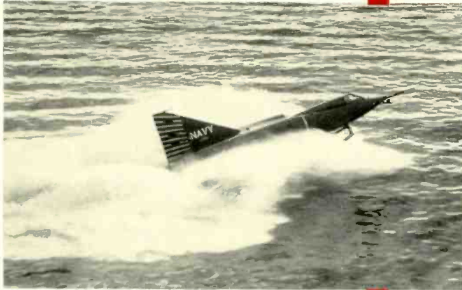
The U.S. Navy's Sea Dart (XF2Y-1) is a sea-based jet plane that takes off and lands on skis.
