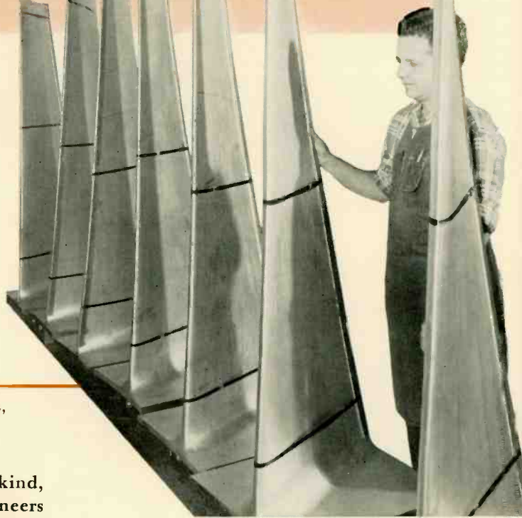
Transonic rotor blades being prepared for shipment. Trailing edges have protective coverings.
