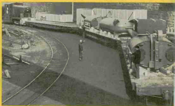
The first of 35 huge 25-million-kva circuit breakers to be built by Westinghouse for Ohio's new 330-kv system.
