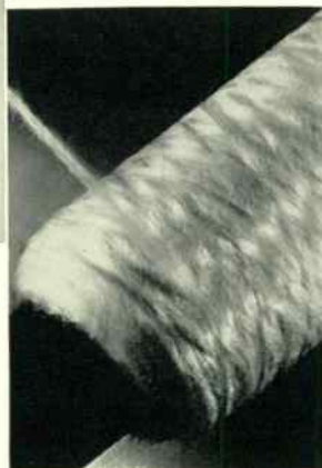
Marbles of glass are melted and flow through orifices forming filaments collected into yarn as shown at right. Photos by the Owens-Corning Corp.
