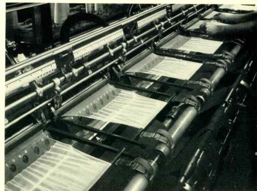
One of the most complex precision-manufacturing devices in all industry is the full-fashioned hosiery knitting machine. Here are 32 "Cameo" brand stockings, in the early stages, being knit simultaneously and automatically in a Burlington Mills factory.
