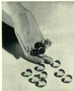
Marbles of glass are melted and flow through orifices forming filaments collected into yarn as shown at right. Photos by the Owens-Corning Corp.
