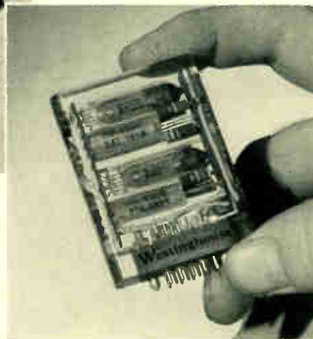
Fig. 6—In production models, instead of using the clear plastic, another inert filler is used that makes the final product opaque. The silhouette shows the relationship of the tiny components of the finished electronic circuit.
