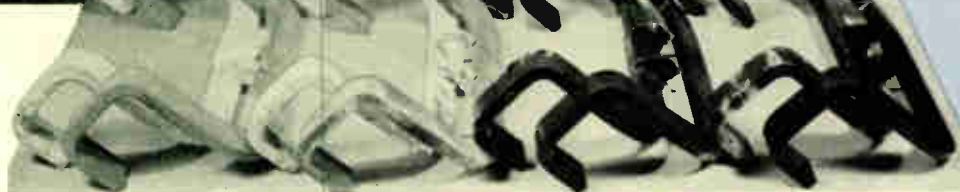
← Fig. 10—Various finishes on hanger irons were exposed to 2000 hours of salt spray. From left to right the finishes are: galvanized; cadmium plated; galvanized and bonderized; cadmium plated and bonderized; galvanized plus mica-base finish; cadmium plated plus mica-base finish; galvanized and bonderized plus mica-base finish; and cadmium plated and bonderized plus mica-base finish. Only the cadmium-plated and bonderized plus mica-base finish hangers (at extreme right) showed no signs of attack.
