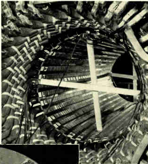
Fig. 7—Two surge-inducing coils are shown in position in the bore of a 3600 rpm generator adjacent to two machine coils for detecting short-circuited conductors.
