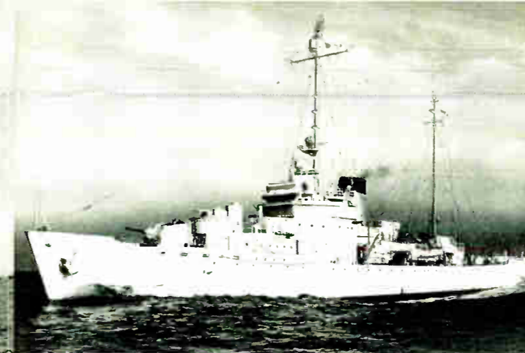
Above is the Coast Guard cutter Campbell . It is the largest of cutters, and, powered with 6200-shp geared turbines, has a range of 8000 miles. At right is the Androskoggin , a turbine-electric ship used in North Atlantic weather patrol.
