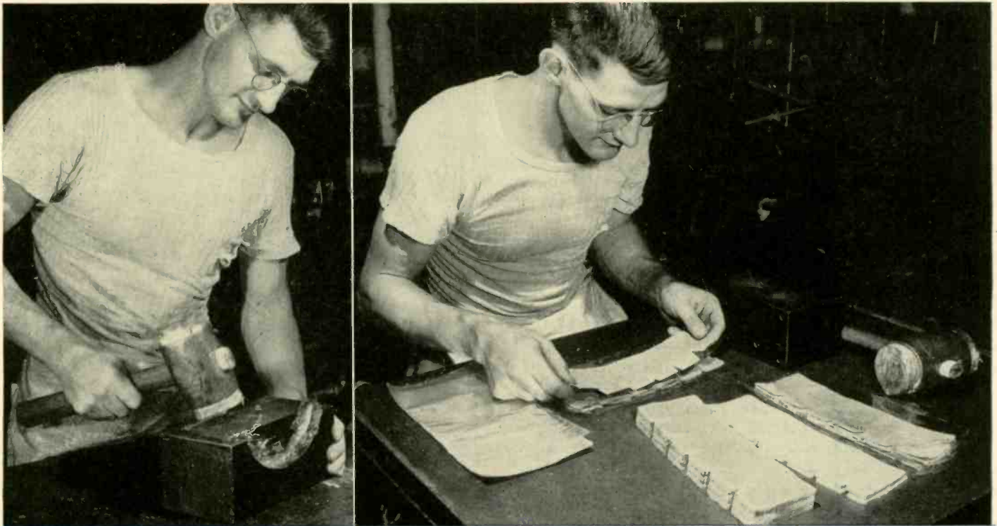
The Fosterite-asbestos material can be made in molded form of relatively complex shapes by building up suitable layers of the impregnated asbestos sheet in a mold and subsequently thermosetting the synthetic resin under heat and pressure.
