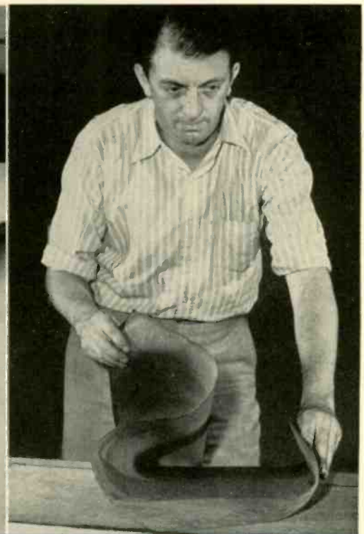
The Fosterite-asbestos material is being made in a wide variety of forms and shapes, from simple flat sheets and rods to molded curved pieces. At right is one sheet of asbestos paper after impregnation with the Fosterite resin, ready for lamination and pressing.
