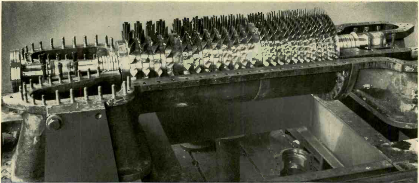
A 30 000-cfm, 6:1 pressure ratio axial-flow compressor with cover removed.
