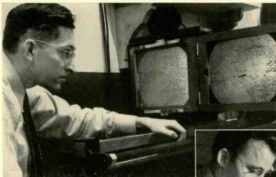
F. C. Hull of the Westinghouse Research Laboratories uses a grain-size comparator. Unknown specimen, left, is matched to standard in illuminated wooden frame. Calibration read from the metallograph gives grain size.
