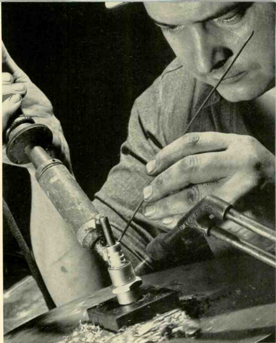
Vacuum-tight seals are necessary for terminal assemblies in high-frequency applications. Here a Zircon porcelain coaxial-cable bushing undergoes a solder-seal operation.
