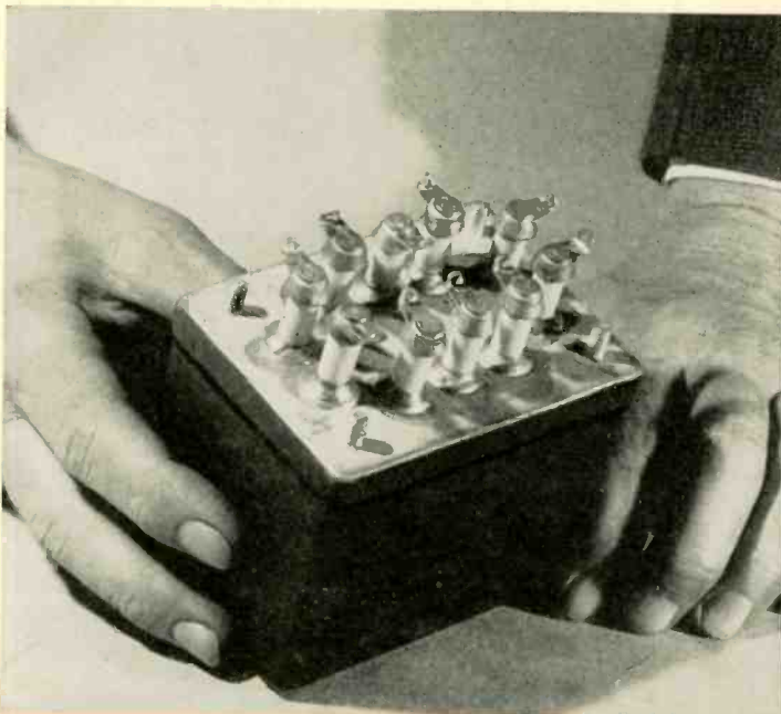
Zircon porcelain bushings, solder-sealed to radar network case-covers, combine not only excellent high-frequency characteristics and vacuum-tight seals but also high shock resistance.
