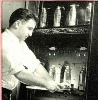
Fig. 3—In the electronic method, the measurements of arc current and voltage are impressed on the grids of thyatron tubes supplying the winch motor. A source of direct current is not required in this scheme. A portion of the panel with tubes in place is at right.
