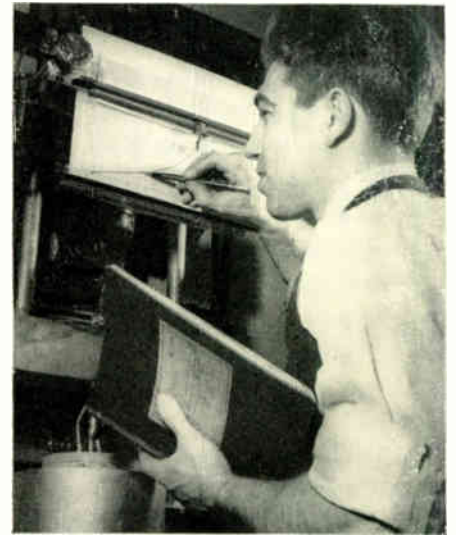
Mr. Manjoine checks the graph automatically scribed by the creep-to-rupture test machine.
