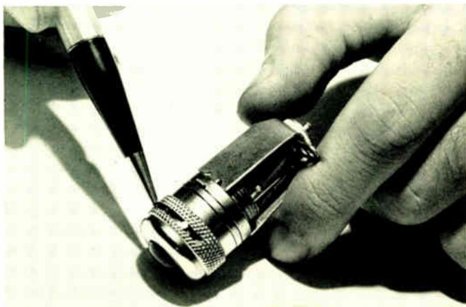
The change in the relative position of two polaroid filters, readily performed by a quarter turn of the knurled ring, permits complete brightness control in this instrument-panel light.
