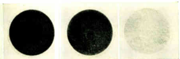
Comparison of blackness spots of equal amounts of air: (left) uncleaned, (center) mechanically filtered, (right) electrically cleaned.
