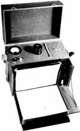
Figure 12. Complete wavemeter with carrying case and calibration charts
