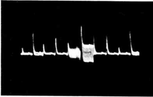
Figure 3. Sending distributor output showing two bands modulated
