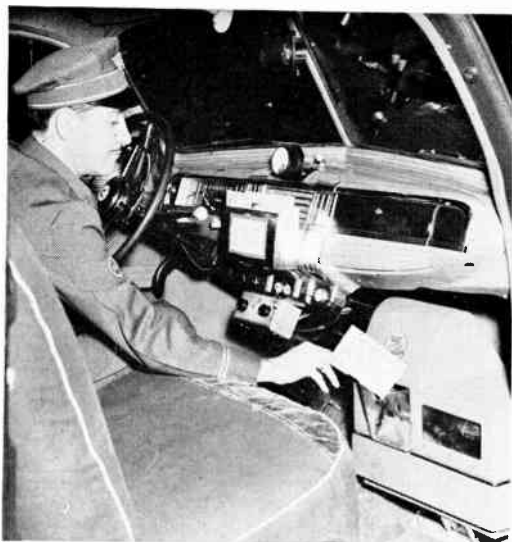
Figure 4. Facsimile recorder as installed in Telecar
