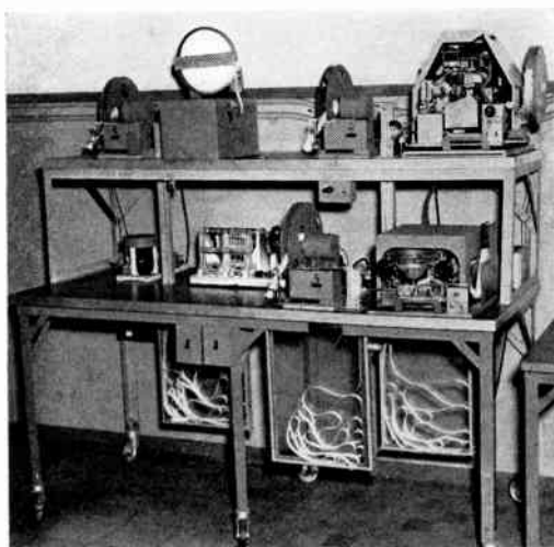
Figure 10. Perforator tape test table
