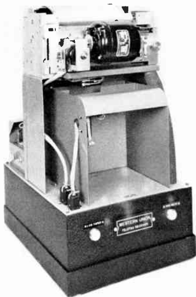
Figure 3. Non-sealing facsimile recorder—cover removed
