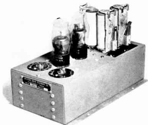
Figure 3. Electronic Timer 105-A—a cold-cathode type which responds to two different timed intervals
