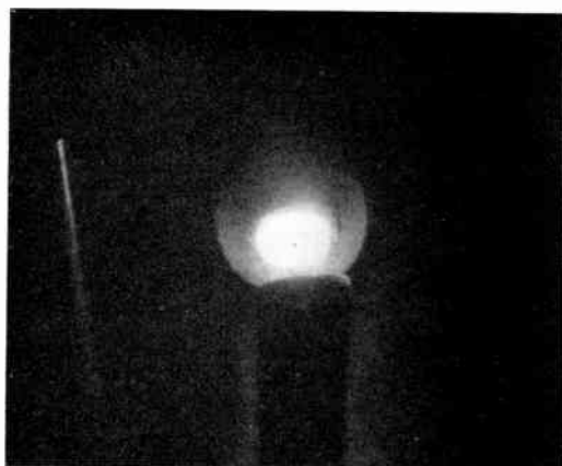
Figure 5. Front view of burning Telcoarc electrodes
