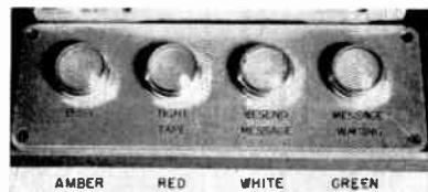
Figure 5. Signal lights at lightly loaded outoffices
