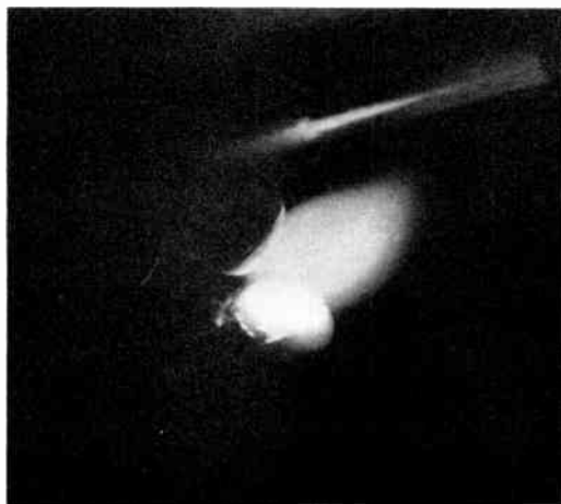
Figure 6. Side view of burning Telcoarc electrodes
