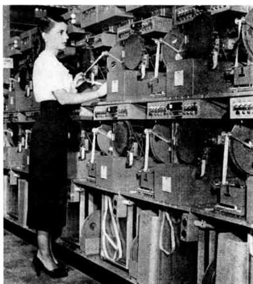
Figure 5. Perforator tape being employed in a Plan 21 receiving position
