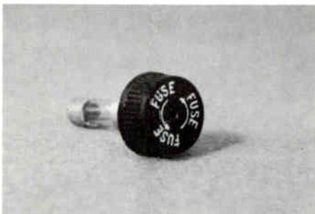
Figure 2. Type 422 Oscilloscope 3-ampere fuse holder with the thin-shell back pierced to allow insertion of a VTVM lead.
