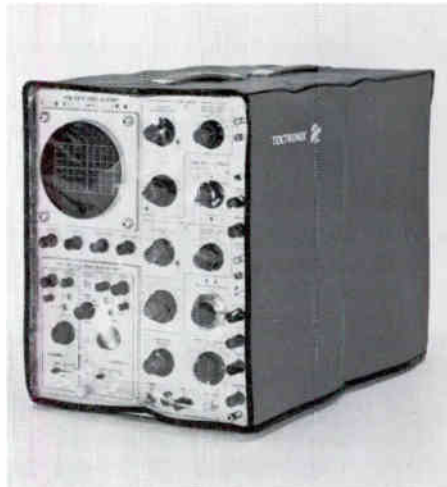
Figure 1. New dust cover for Tektronix oscilloscopes shown on a Type 545B Oscilloscope.
