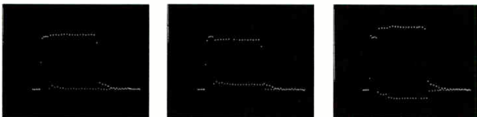
Fig. 6. Waveforms of: (a) correct DTR, (b) low loop gain, (c) excessive loop gain, using a small charge line on one side of the switch and none on the other.
