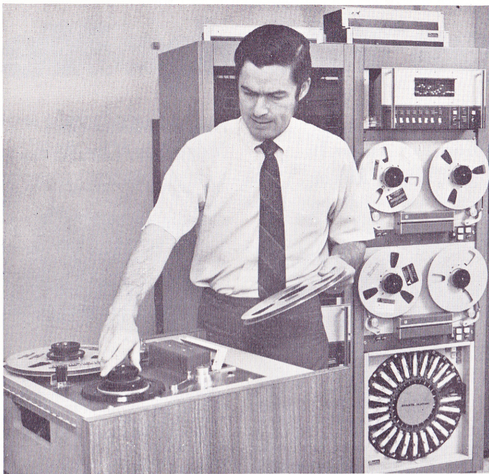
SPARTA-MATION systems are designed to accept a station's present tape equipment. Here, Dave Evans loads a music tape on a Teac R-310 which connects to the system in the background.
