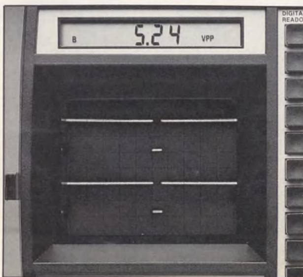
Fig. 5: The scan lines for the front panel switches were checked with the SC61 to find out which line was being fed through a switch. It was then a simple matter to verify that the eject switch was defective.
