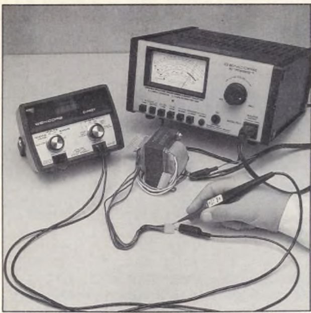
Fig. 3: The best test for power transformers is to measure the voltage of each of the output windings.
