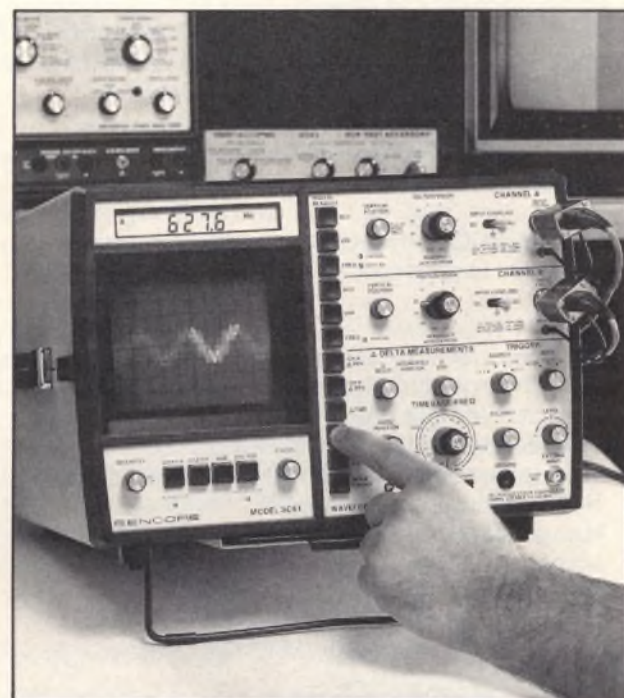
Fig. 10: The delta feature of the SC61 lets you measure the frequency of the downconverted chroma signal.
