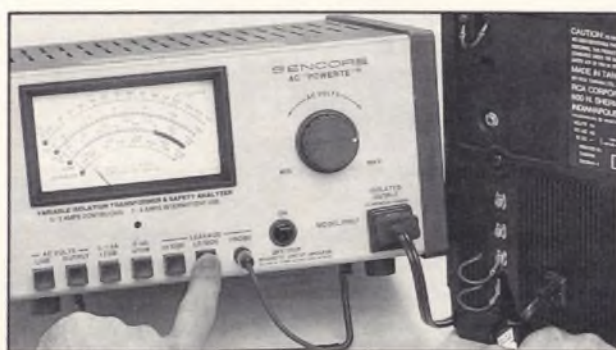
Fig. 1: To make a safety leakage test with the PR57, simply plug the chassis into the POWERITE and touch the probes to any exposed metal surfaces.
