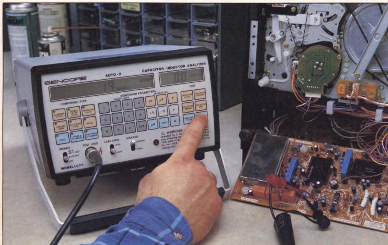
Fig. 3: Simply connect the leads and press a button. The patented LC77 Ringer test shows a number greater than 10 if a coil is good, or less than 10 if it is bad, even in the circuit.
