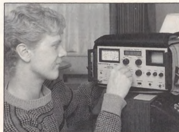
Fig. 6: The FS74 TV-RF Signal Analyzer proves that the cable is the problem. The servicer can now concentrate on solving "in house" cable problems or confidently advise the cable company.
